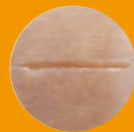
Super-Pulse mode pulse duration=10µs
