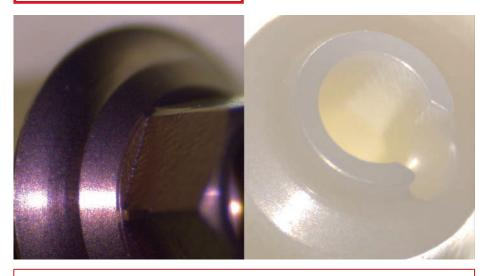
The **matrix®** interface milled in a local dental lab shows the same precision and surface quality compared to a TRI® abutment manufactured in Switzerland.
