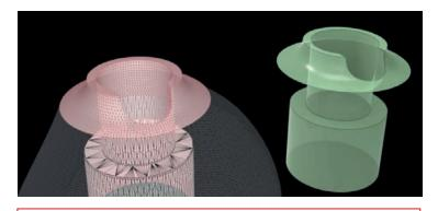
The interface of the crown and the screw seat is replaced with a high-resolution CAD file.
