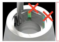
Conventional connection are designed to be manufactured with industrial production machines. Sharp edges cannot be milled with standard dental milling machines.
