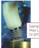
Sample I.D. BL-15 Max Load 463 N at 12.300 cycles
