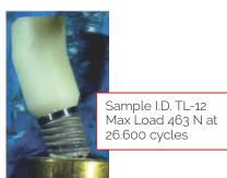
Fatigue Test Failure Mode - Implant crack below pot line
