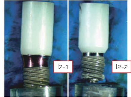
Post Fatigue - No failure at 2.000.000
